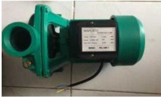
*Gambar 8. Pompa Air Baru*
