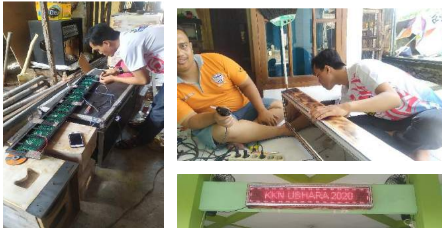
Gambar 20 dan 21 : proses perakitan alat promosi berbasis digital ( Running Text Electronic )
